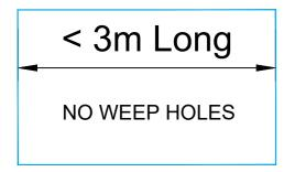
Planks < 3m, water can easily flow out of the cores during the various stages that the plank is in transition. On this basis weepholes are omitted. Plank length affects the arrangement of weep holes
