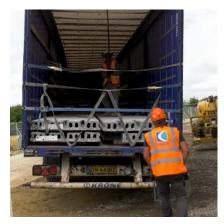
The slinger/banksman will open the rear doors and roof of the trailer. Ratchet straps can be used as edge protection.
